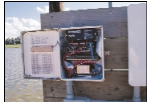
Though pond-condition data can be viewed and controlled via a personal computer, special display-equipped enclosures (shown open above) also make data visible on-site.
