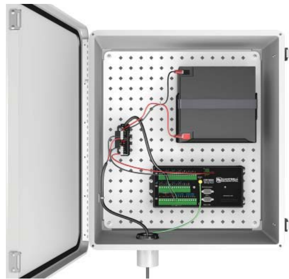
An enclosure with the -SC option includes one 1.5-in diameter port for cable entry. Shown is an ENC16/18 housing a CR1000 datalogger and BP24 battery pack.
