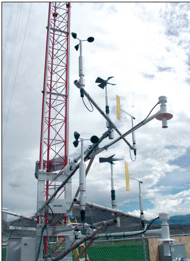
Going up? Preassembled instrumentation platforms await deployment on electrically powered lift carriages.
