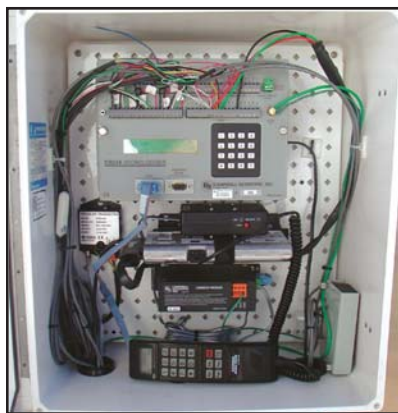
The ENC 16/18 enclosure functions as an "on-site headquarters;" the CR23X enables quality control, performs data calculation, and provides communications through a COM200.
