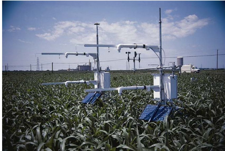
FIGURE 2-1. ASPTCs Mounted to Bowen Ratio Arms
