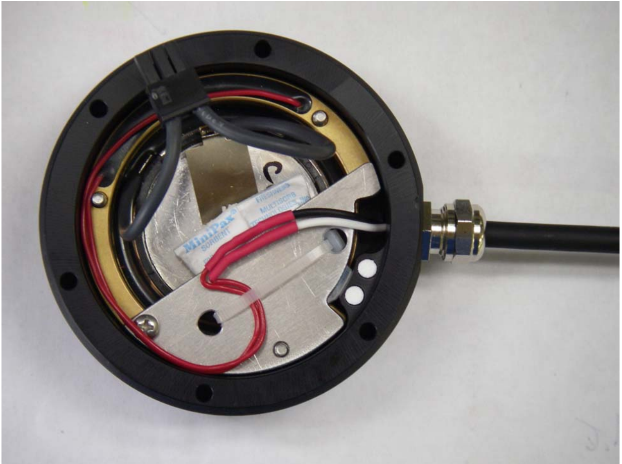
Figure 15 Complete transducer assembly with power connection
