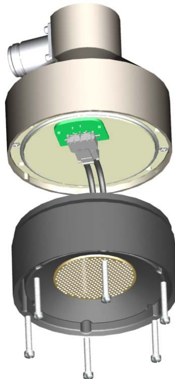
Figure 10 Remove transducer housing and disconnect wires
