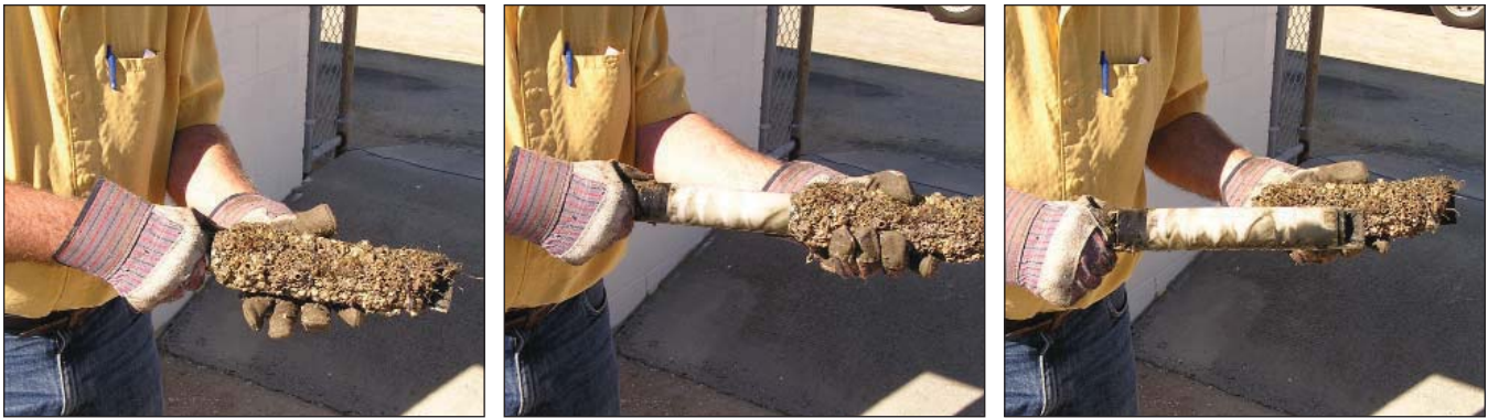
The OBS500 has a plastic sleeve option that can simplify cleanup. The three above photographs shows the sleeve being removed.
