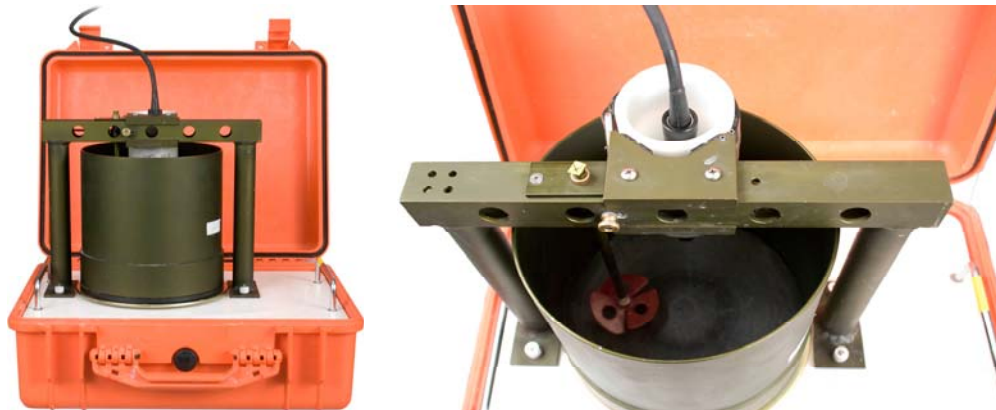
FIGURE 4-4. Portable Sediment Suspender (left) and OBS Beam Orientation in Suspender Tub (right)
