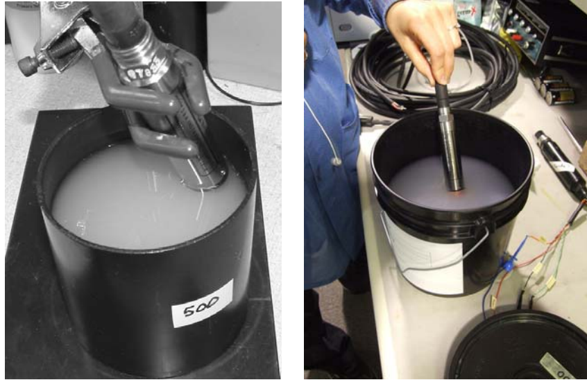
FIGURE 4-3. OBS-3+ (left) and OBS300 (right) in 500-NTU Amco® Clear Turbidity Standard in 100-mm Black Polyethylene Calibration Cup
