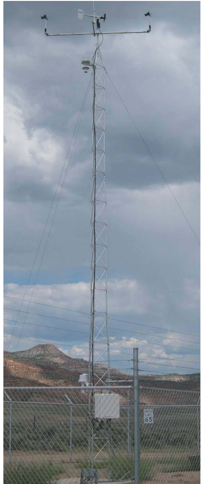
A CM206 crossarm is mounted atop this UT30 30 ft tower. On each end of the crossarm, a CM220 bracket is used to attach a 27106T vertical anemometer. Two 43502 Aspirated Radiation Shields are also fastened to a leg of the tower.
