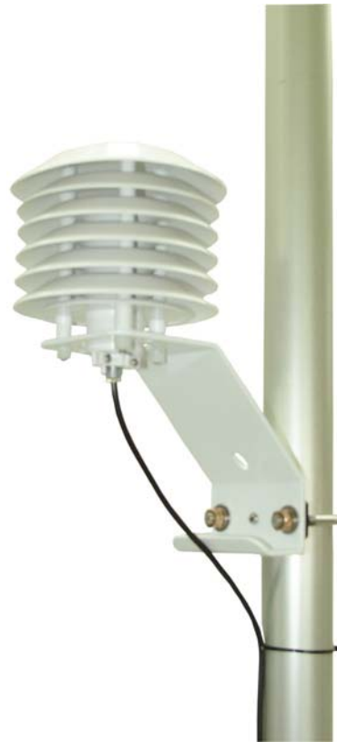
FIGURE 1. HMP50 and 41303-5A Radiation Shield on a Tripod Mast
