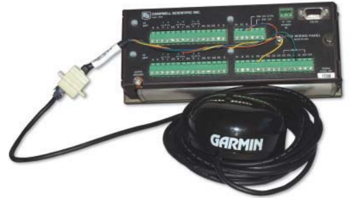
An RJ45 Interface Cable connects the sensor to the datalogger's control ports. This interface option is compatible with our CR800, CR10X, CR1000, and CR3000 dataloggers.
