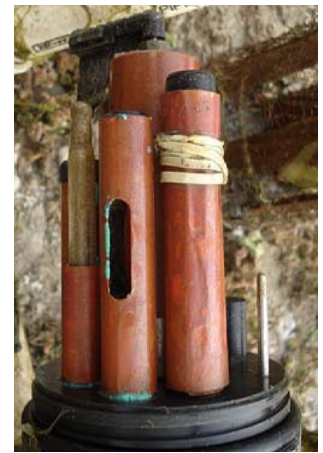
Above: sensors fouled after deployment (l) vs. sensors deployed with copper tape (r)
