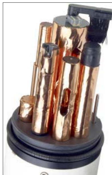
Above: sensors wrapped with copper tape
