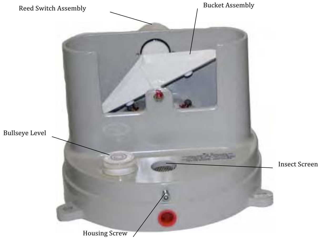
FIGURE 7-1. Components of CS700 Base
