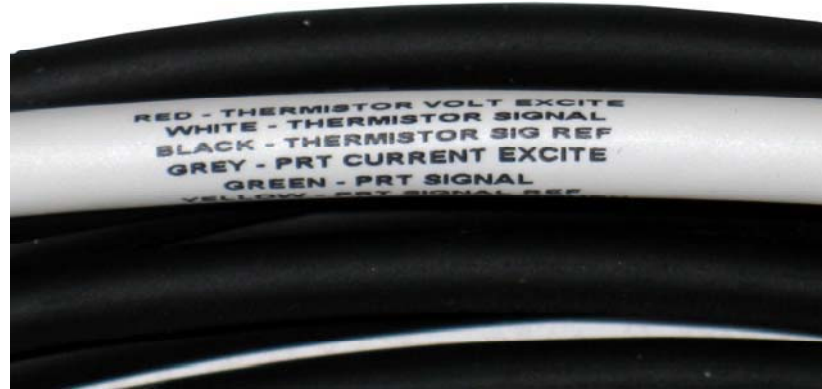
FIGURE 6-4. Labels on the pigtail end of the TEMP cable.
