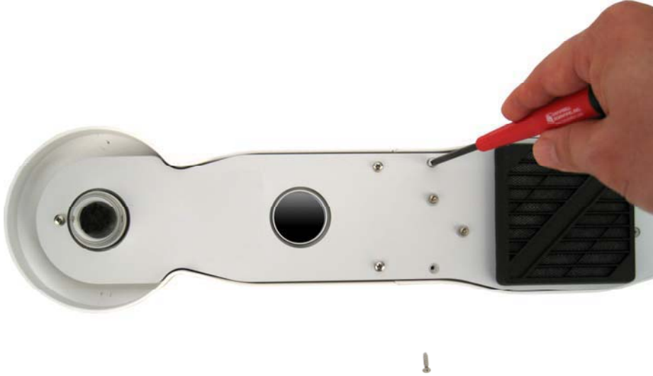
FIGURE B-5. Attaching the solar shield to CNF4 using four flat-head screws.
