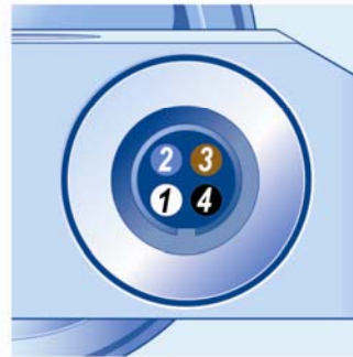
FIGURE 5-1. Pin Layout on Campbell Scientific Black Cable
