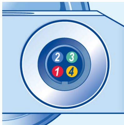
FIGURE 5-2. Pin Layout on Kipp & Zonen Original Cable
