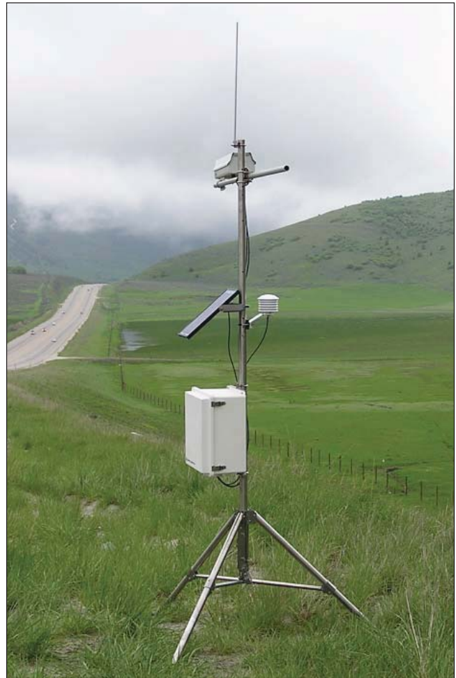
The CM110 10-ft tripod shown above is not guyed. An optional guy kit is offered for the CM110 if additional stability is required. A guy kit is shipped with the CM115 and CM120.
