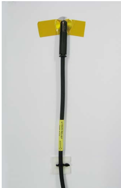
FIGURE 3-3. 110PV mounted to a PV module using Kapton tape
