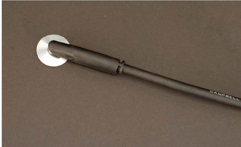
FIGURE 3-1. 110PV mounted to a PV module
