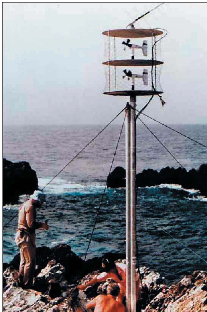
An innovative method of discouraging interference from birds is shown in this photo of a wind measurement station at St. Peter and St. Paul Rocks (Brazil). The station was located in the mid-Atlantic during the SEQUAL (Seasonal Equatorial Atlantic Experiment) field program. Photo courtesy Dr. Silvia L. Garzoli (Director of the Physical Oceanography Division of the Atlantic Oceanographic and Meteorological Laboratory of NOAA).
