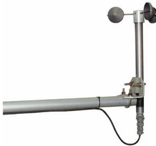
FIGURE 3-2. 014A Mounted on a CM200 Series Crossarm with CM220
