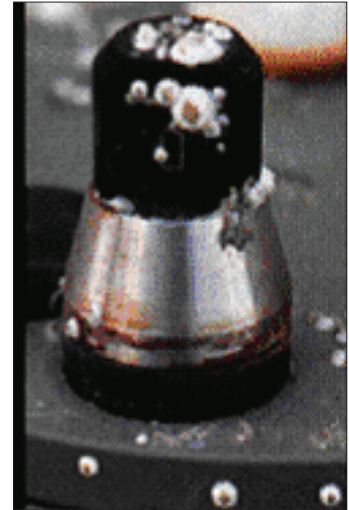
Figure 3. The barnacles on this OBS sensor produced erroneously low turbidity readings.
