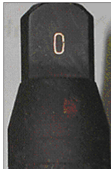
Figure 1. An OBS sensor fouled with a tannin-based film.
