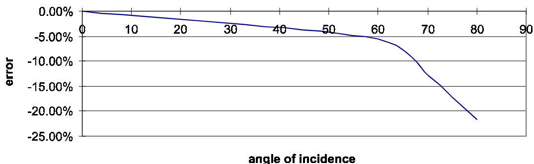
FIGURE 4. Cosine Response of a Typical Net Radiometer
