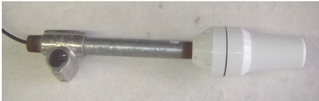
Figure 27: Antenna Attached to Mount
