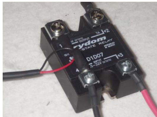
Figure 36: SYN-DC-936R & Relay Connected
