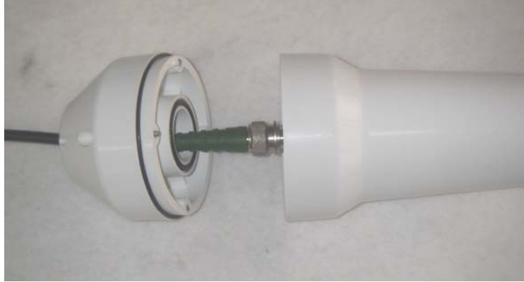
Figure 26: Antenna and Cable Connected
