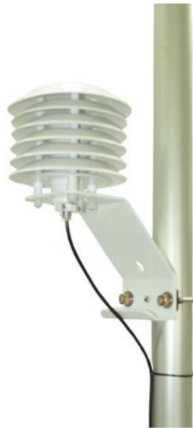
FIGURE 2. HMP60 and 41303-5A Radiation Shield on a Tripod Mast
