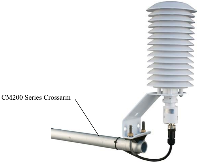
FIGURE 3-2. HMP155A and 14-Plate Radiation Shield on a CM200 Series Crossarm
