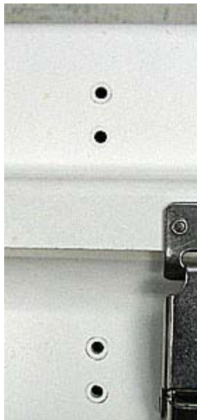
FIGURE A.1-6. The proper placement of the screw holes are shown in a close-up (left photo) and distant view. Ensure that the screw holes for both brackets are aligned with each other.
