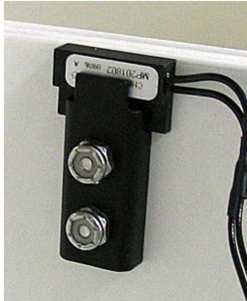
FIGURE A.1-3. Switch installed in the enclosure case.
