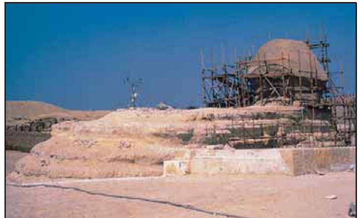
Weather measurements on the Sphinx provided input for its preservation, Cairo, Egypt.
