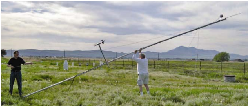
FIGURE 2.5-1. Raising the Mast
