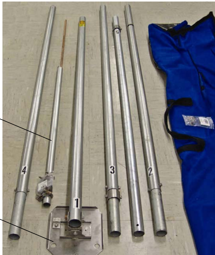
FIGURE 2.2-2. Mast Sections and Base
