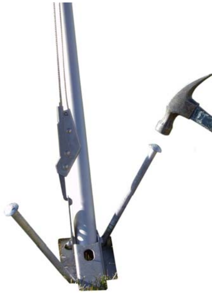
FIGURE 5-10. Staking the Tripod Feet
