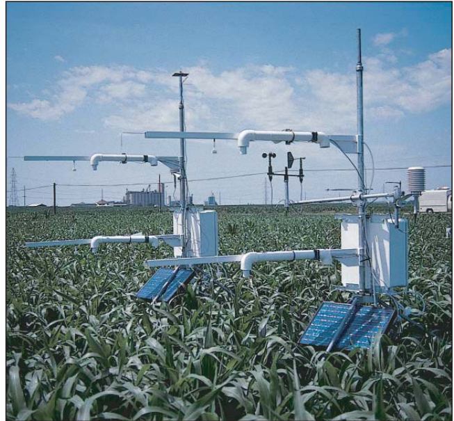
These Bowen ratio systems at a sorghum field near Lincoln, Nebraska include ASPTCs attached to the upper and lower Bowen ratio arms.
