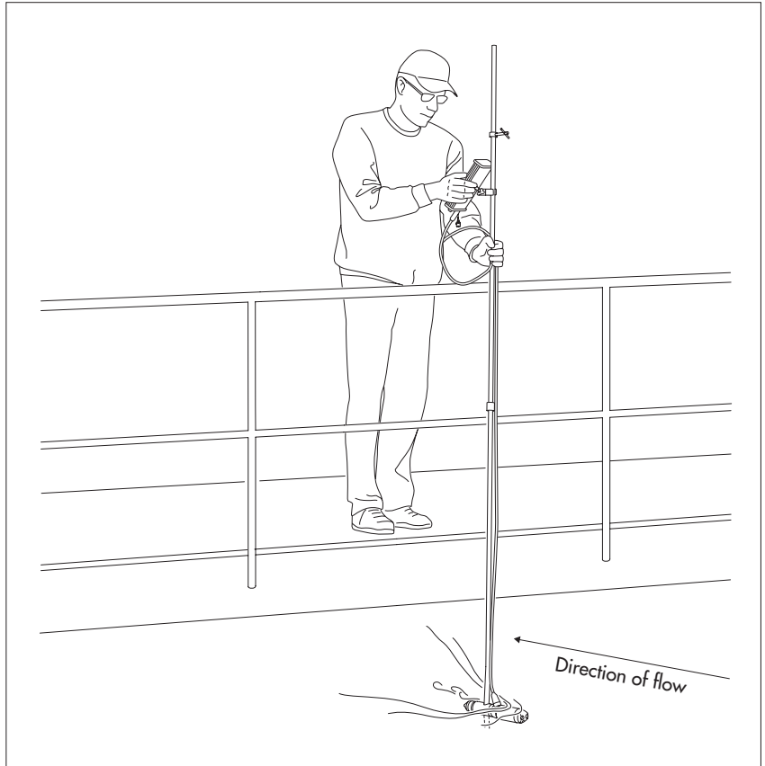
Fig. 13: Positioning of the OTT ADC sensor in the water
